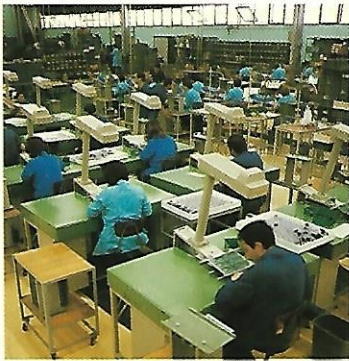
Computer-helped manual components assembling.
