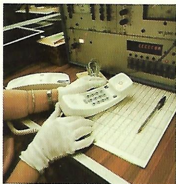
Final telephone set test.
