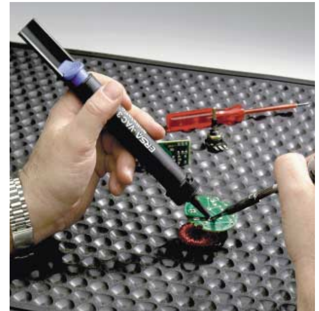
Removing heated and melted solder by means of a mechanical desoldering pump
